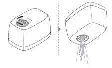
Press the protruding part of the connector to extract the remaining water.
