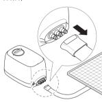
Remove the cap by turning it counterclockwise and tilt the heating unit to remove the water and empty the heating unit.
