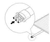
Pold the pad and remove the residual water inside. Connect the air pump into the center of the removal kit and pump until no water comes out.
